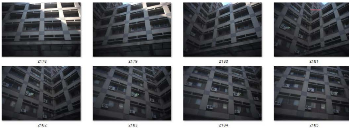
Figure 11. Test images taken with the non-metric camera Basler A102kc on an MMS
